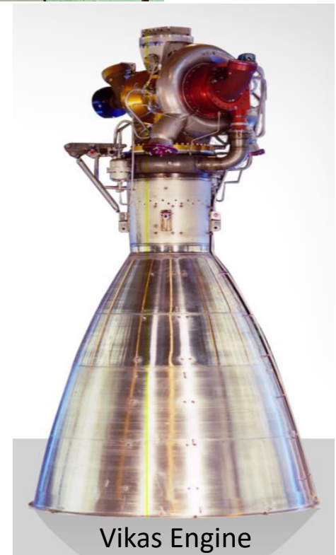
THRUST CHAMBER VIKAS ENGINE USED FOR CHADRAYAN.
