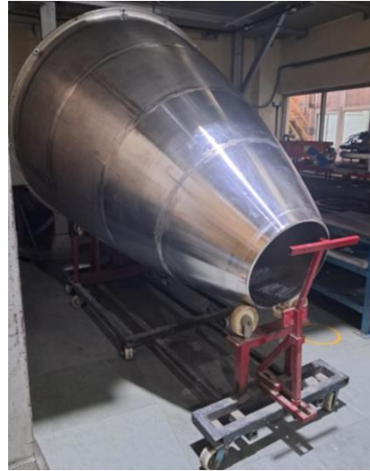
VIKAS ENGINE DIVERGENT ASSEMBLY DONE WITH ROLLING FORMING AND EXPANSION PROCESS OF CONES.
