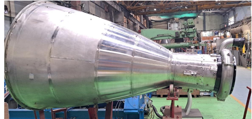
THRUST CHAMBER VIKAS ENGINE USED FOR CHADRAYAN.
