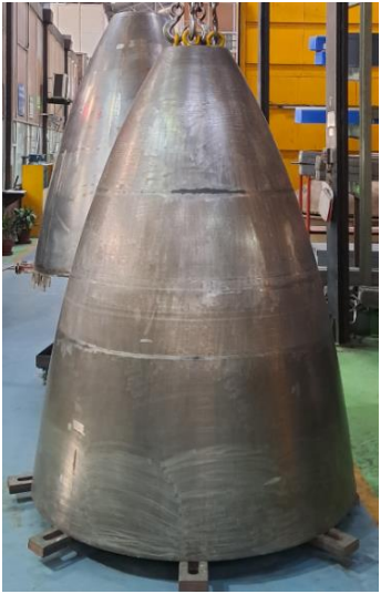
PUNCH USED FOR 90% FORMING OF CONES. 100% FORMING IS DONE ON EXPANDER.
